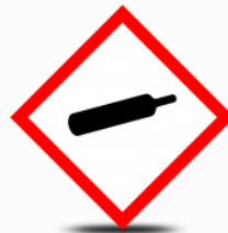
Compressed Gas Hazard
